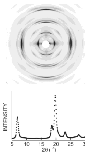
Figure 3. X-ray diffraction pattern and equatorial profile of \beta -chitin– p -phenylenediamine complex prepared by treating \beta -chitin hydrate with 1% (w/w) p -phenylenediamine/ethanol solution.
